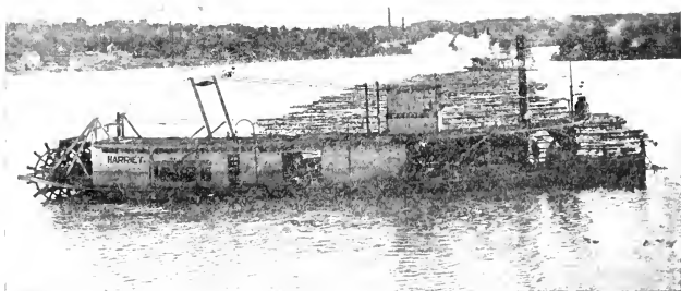
FIG. 149. — A Mississippi River Log Raft, Showing the Method of Control by End-wheeled Steamers.
